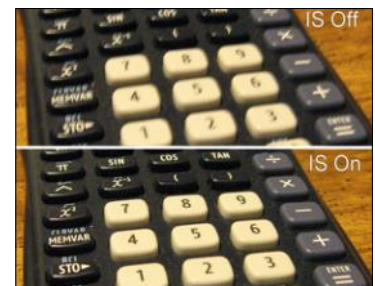
A comparison of close-up photographs of a keypad with and without IS.
